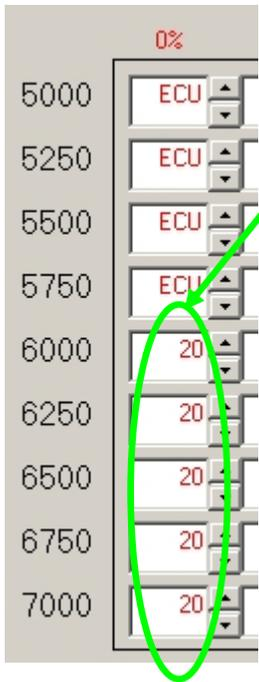
ECU runs huge timing advance after high RPM shift. This can cause knock after shift conditions
